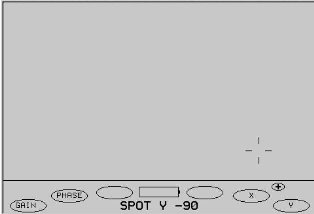
The cross-hairs allow the operator to observe if the balance point has drifted or moved due to an artefact or material condition.
