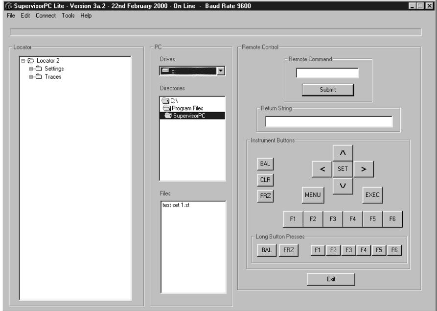
The remote control function operates by the simulated keys on the right hand side of the screen. These can be used in place of the keypad to control the instrument.
