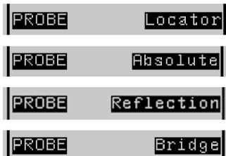
Probe type can be set to Locator, Absolute, Differential (Bridge) or Reflection.
