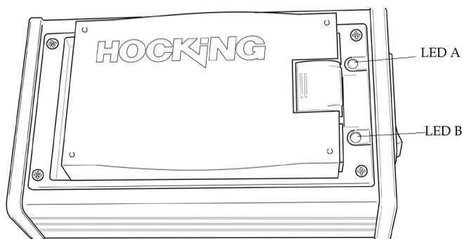
The battery charger/eliminator should be connected an AC supply using an appropriately terminated plug. The adapter is able to switch to power supplies that are in the range of 90 to 264VAC, and 47 to 440Hz. Once the unit has been connected the mains switch on the side of the unit should be switched on.
