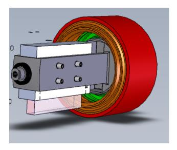
Note the vertical position of the array in this picture is incorrect, the array face should be flush with the axle.
