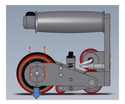
Press the wheel probe firmly on a flat surface, and adjust the angle of the axle to obtain the maximum amplitude echo. Use an Inspection Gate to monitor the amplitude of the echo.
