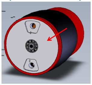
Gently pull the end plate away from the assembly. Do not twist the plate or use force to remove, as this may cause damage to the small bearing and seal.
