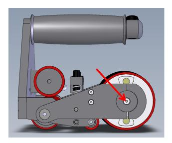
This fastener can be stiff, apply copper grease on re-assembly. If in doubt replace with a new fastener. Do not completely remove the fastener at this stage.
