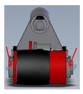
Do not fully tighten the four cap head fasteners at this stage
