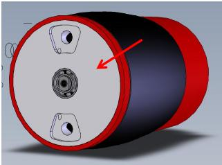
Fit the side plate onto the axle, taking care not to damage the small bearing and green seal as it fits over the end of the axle. Press the side plate firmly against the tyre.
