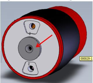
Fully remove the countersink fastener, and remove the retaining disc from the axle.
