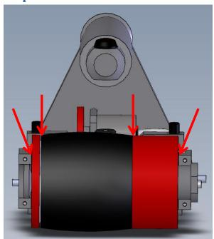
Step 12: Mount the roller into the buggy assembly
