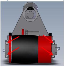
Undo the 4 fasteners shown, remove them and remove the two C clamps.
