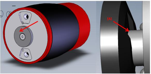
Check that the slot in the disc aligns with the slot in the axle (A).
