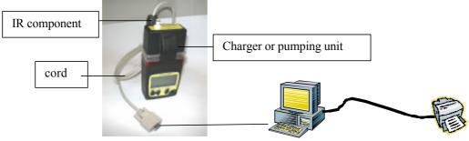
2) MX 2100 integrated in a "Twincall" calibration station which is, itself, connected to a computer and a printer.
