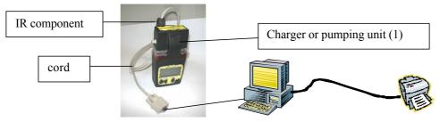
(1) A charger or sampling unit can be used to mechanically hold the IR cord on the appliance.
