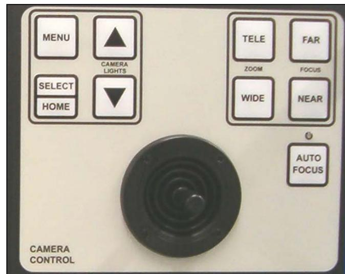
The on-screen menu system is navigated using the group of four buttons to the upper left of the camera control joystick. Many items in the menu can also be accessed and / or activated using keyboard hot-keys. General navigation using the panel buttons is as follows:
