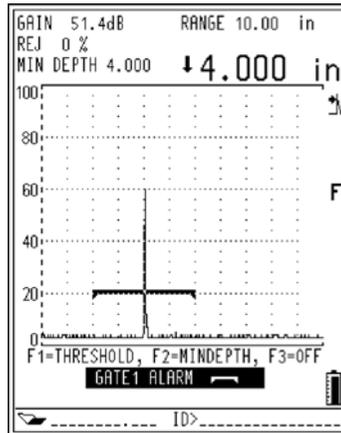
Figure 5-4: Negative Logic Alarm
