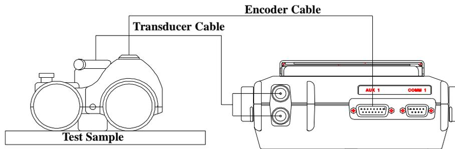
**Figure 9.3:** Epoch III B-Scan Setup Diagram
