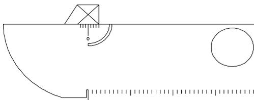
**Figure 4.16:** Location the Beam Index Point
