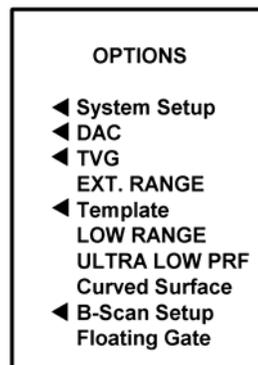
To select a particular item, use the **[←]** and **[→]** slewing keys to move the highlight bar up or down the list to the desired item and press **[ITEM SELECT]**. When an item has been selected, the appropriate Set-Up Menu will appear. For example, to review the basic system set-up, the following sequence is used:
