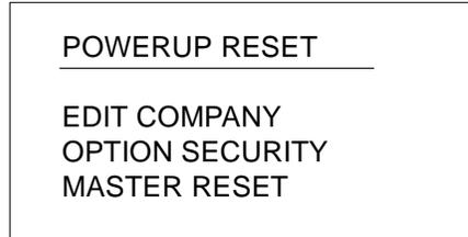
Use the **[←]** and **[→]** slewing keys to position the highlight bar over “EDIT COMPANY” and press the **[ITEM SELECT]** key. The Epoch III will progress to the Power Up screen. You will notice that there is a flashing cursor next to the address field in the middle of the display. The size of the field is 5 lines of 33 characters each. F prompts (F1, F2, F3) appear along the bottom of the screen.
