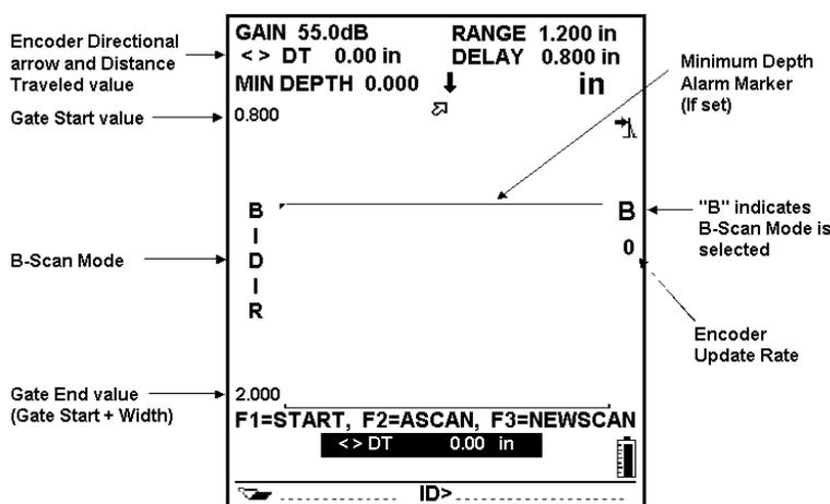
**Figure 9.4:** Bi-Directional B-Scan Start Screen
