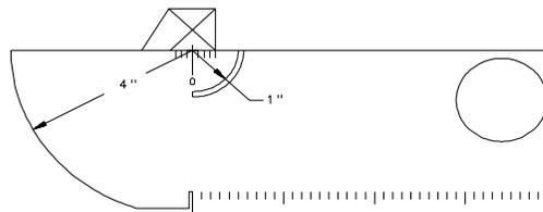
**Figure 4.18:** Calibrate for Distance
