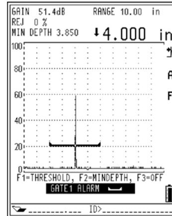
Figure 5-5: Positive Logic Alarm
