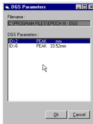
A calibration can be opened in the Interface Program after it is uploaded from the EPOCH III. The DGS curve is not visible, but the DGS parameters can be verified or adjusted as necessary. Click **File**, then **Open**. Select the file to be opened, then click **[OK]**. If multiple IDs have been saved in the file, a prompt box will be displayed asking the user to select the appropriate ID to open.
