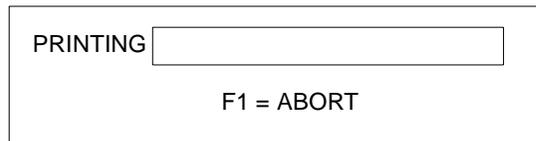
The bar graph next to “PRINTING” shows approximately how much of the data has been sent. Since the size of print buffers vary, this will determine the time necessary for the Epoch III’s keypad to return to normal.
