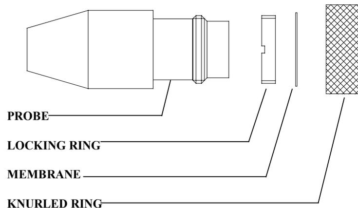
**Replacing the Membrane in the Knurled-ring**
