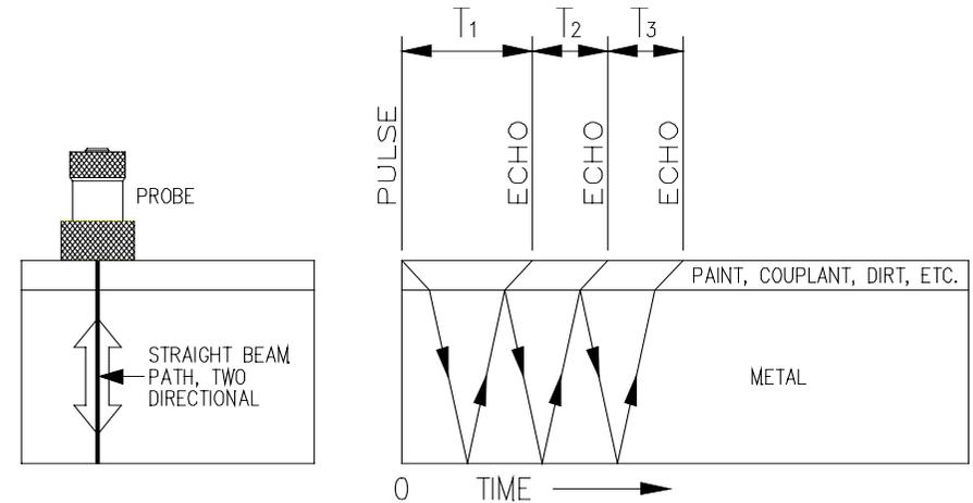
The *multiple-echo* beam travel is depicted above, spread out for time, to illustrate the timing method. The beam path is in fact straight, at 90 degrees to the surface and the ultrasonic energy reverberates up and down within the metal (as shown in the small sketch above - left). Each time the echo is reflected back down, a small portion of the energy comes up through the coatings, striking the Probe which now acts as a receiver.
