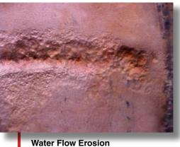
Water Flow Erosior 7 mm Plate
