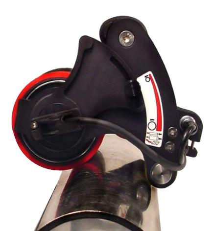
cally for Longitudinal scanning. On pipe diameters of less than 24 inches/60 cm, this accessory improves stability by supporting the WheelProbe tyre, allowing you to obtain the best results from the WheelProbe over a greater range of pipe diameters.
