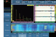
OmniScan MXU software displaying C-scan view of corrosion.
