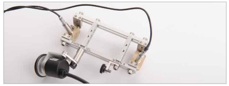
WREN 4 - Weld Root Erosion Scanner
