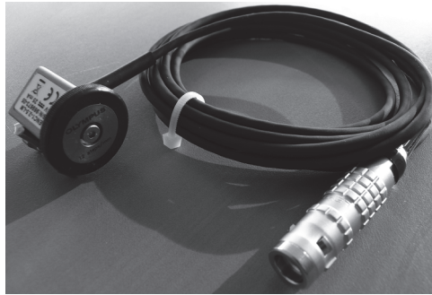
Figure 1-4 The Mini-Wheel encoder and cable
