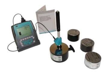
Equotip test blocks are delivered calibrated with the impact device that the customer uses to check his metal parts, e.g. in HLD, HLDL, HLE. This means that the calibrations are precise and are not based on conversions. Calibration certificates are issued by Proceq (factory calibration) or an accredited institute (national traceability), as per customer request.
