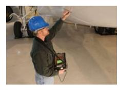
On-wing, wide-area scanning with arrays ensure complete inspection coverage of aluminum and composite structures.
