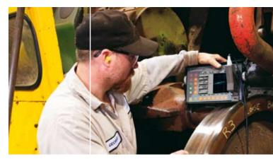
Specially designed transducers allow wheel inspections to be carried out faster, still providing more reliable results.
