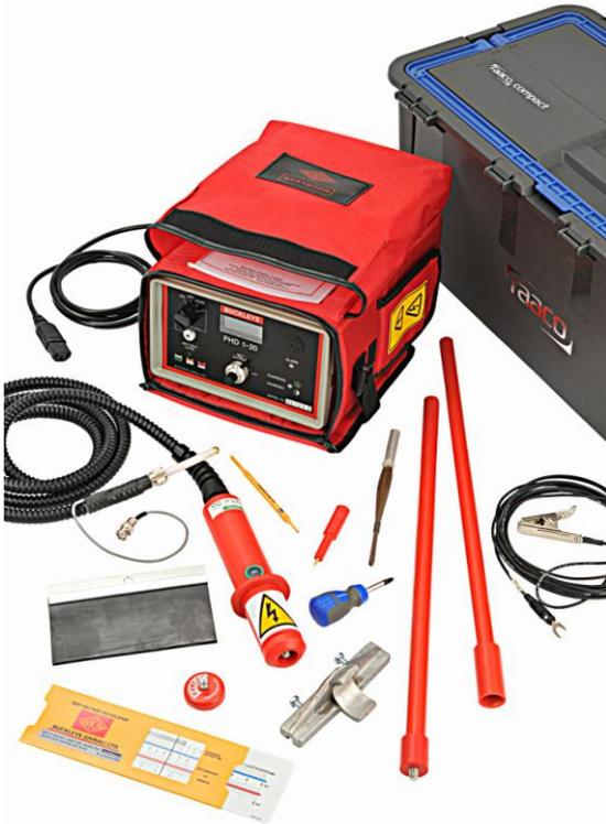
Buckleys Pinhole / Holiday Detectors enable inspectors to check quickly and effectively for porosity, pinholes and other faults in a wide range of non-conductive coatings and linings.
